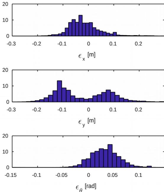
Fig. 3 – Histograms of the uncertainties in position and orientation measured by the embedded vision system installed on the *Friwalk*.
