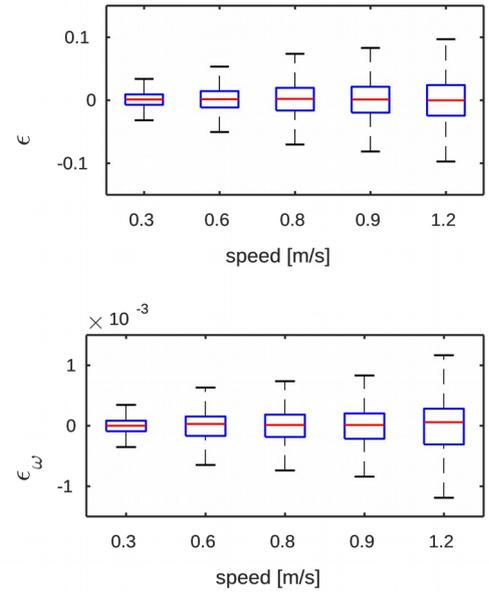
Fig. 2 – Box-and-whisker plots of the uncertainties in linear and angular speed measured by wheels encoders.
